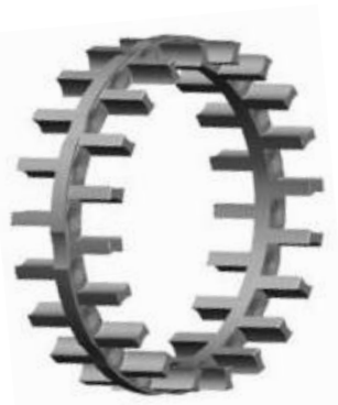
Fig. 5. One-piece finger-type cage.
