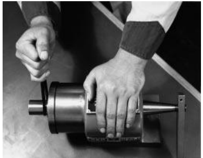
Figure 7 – Tightening with Spanner Wrench
