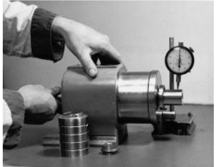
Figure 6 – Checking Nose-End Runout
