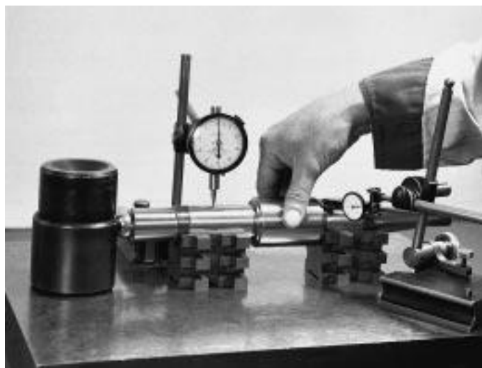
Figure 2 – Inspection of Shaft
