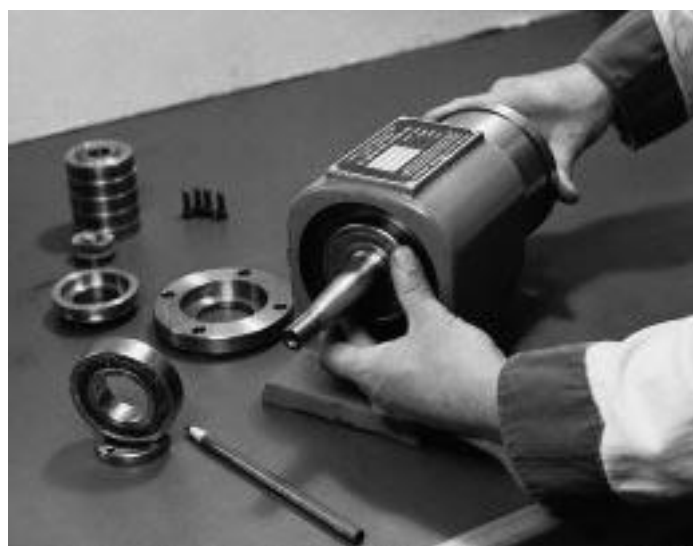
FIGURE 5 – MOUNTING DRIVE-END BEARINGS
